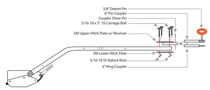
\*\*DO NOT TIGHTEN HITCH PLATE BOLTS UNTIL SUB-FRAME IS INSTALLED\*\*
