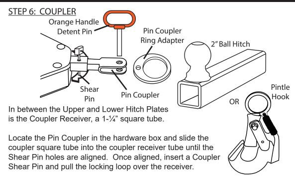
If installing on a 2" Ball or Pintle Hook, place the Pin Coupler Ring Adapter over the 2" Ball or on the hook. Slide the small hole on the Ring Adapter between the upper and lower tabs of the Pin Coupler. Insert the Orange
