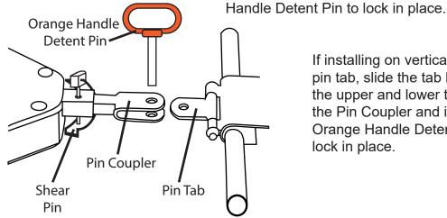
If installing on vertical swivel pin tab, slide the tab between the upper and lower tabs of the Pin Coupler and insert the Orange Handle Detent Pin to lock in place.
